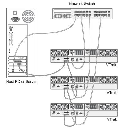
Figure 18. VTrak E310s cascaded management and data connections
